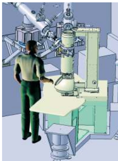
Platform for integration in double/clean room floors with additional mass for the reduction of vibration peaks
