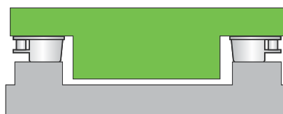
Vibration insulation concrete block or steel platform
