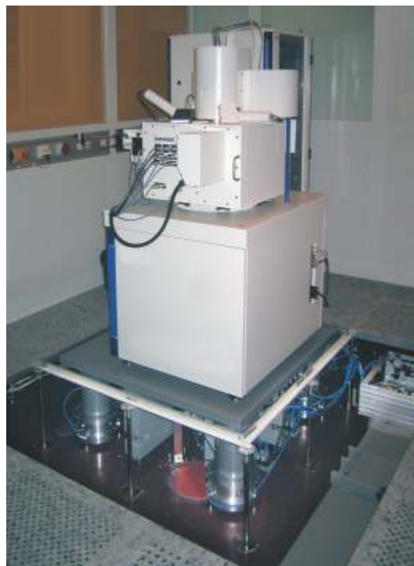
Platform for integration in double/clean room floors with additional mass for the reduction of vibration peaks
